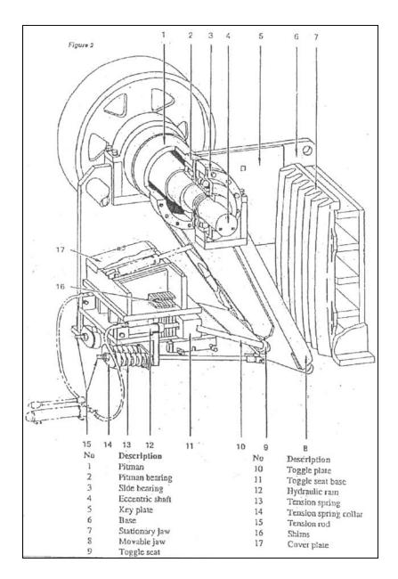
Aplt. App., Vol. 11 at 2389. When material enters the crushing chamber, it is crushed by two jaws, one stationary (labeled "7" in the diagram) and one movable (8). The top of the movable jaw, powered by the pitman (1), follows a circular path with a diameter of 1¼ inches, closer to and then farther from the stationary jaw. The cyclical compression
