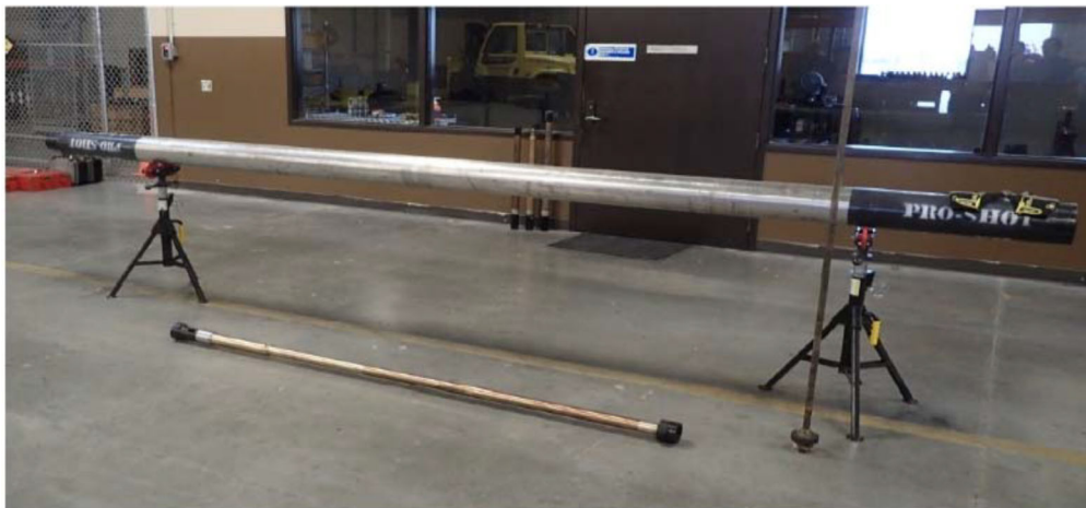
Figure 3: Exemplar Teledrift ProShot (on floor) and sub or drill collar (on stand)
