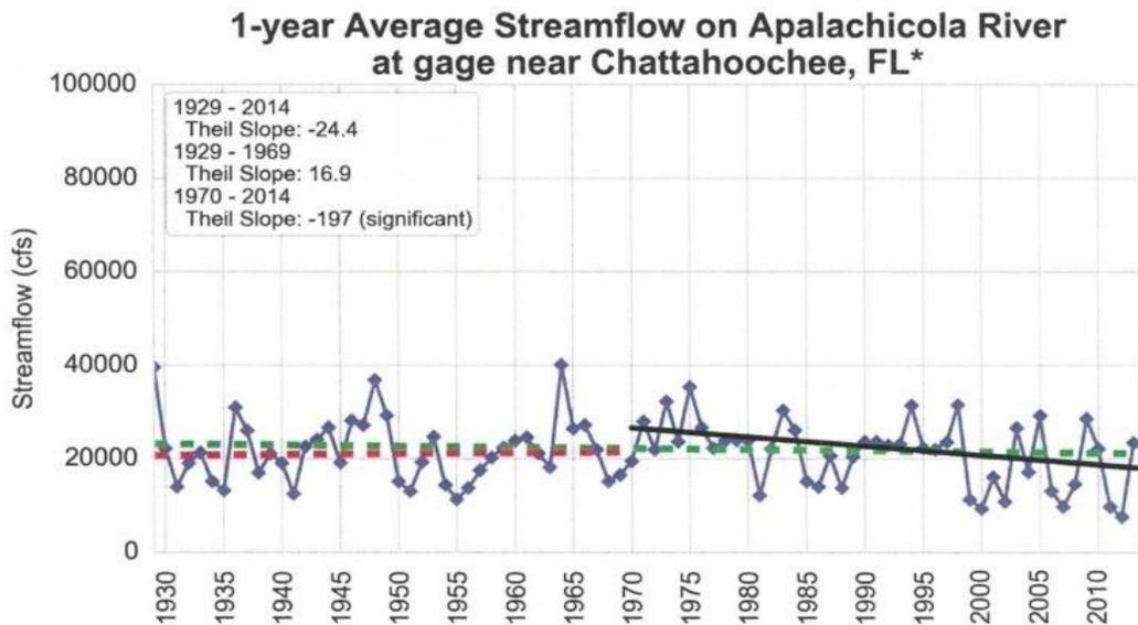
**Figure 9. Annual streamflow trends at the Apalachicola River Chattahoochee Gage using the Theil Slope estimator (Exhibit F565).**
